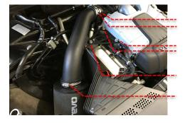
For CREC engine vehicles take the Revo 90° hose connector and fit to the vacuum pipe near the throttle body. Next, take the 6mm vacuum hose that is supplied with the kit and fit one end to the 90-degree connector and the other end to the take-off on the underside of the intake pipe.
