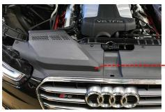
19 Clip the OE intake ducting into the heatshield and into the front air intake.
