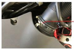
7 Remove the airbox from its mounts by pulling firmly upwards. Do not remove completely yet as the breather hose is still connected on the underside.
