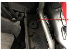
15 Remove the T25 bolt from the back of the headlight.
