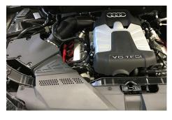
2 Using a T30, remove the 4 x bolts along the slam panel and then pull free from the 6 x clips along the front edge.
