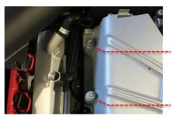
Take the Revo bracket (supplied) and place over the 2 x supercharger studs. Next, secure the intake pipe to the bracket using the supplied M8 x 20mm bolt, 2 x M8 washers and M8 nylock nut. Refit the 2 x supercharger nuts but do not tighten fully yet.
