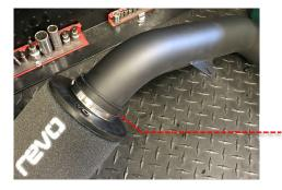
Press the filter and intake pipe assembly in to the Revo intake coupler hose and position correctly in the engine bay. Do not tighten the 3 x hose clamps fully yet.
