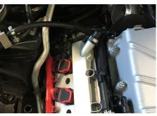
Take the Revo breather filter (supplied) and press into the breather hose until it clicks into place. Next take the P-clip (supplied) and place around the breather hose. Secure the P-clip to the Revo bracket using a M6 bolt, M6 washer on either side of the P-clip and a M6 nylock nut. Do not tighten fully yet.
