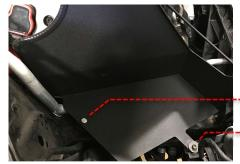
18 Refit the front air intake and slam panel.
