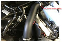
23 Using a 13mm socket, remove the 2 x nuts closest to the throttle body securing the supercharger.
