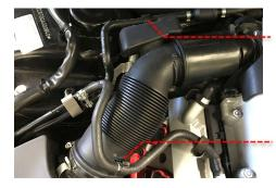
6 Using a 7mm socket, loosen the hose clamp on the airbox end of the intake pipe and remove the pipe from the airbox.
