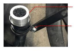
12 Remove the T25 bolt securing the OE airbox mounting bracket. This bracket can be placed out of the work area.
