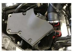
Bisconnect the breather hose by squeezing the tabs and pulling the hose free. The airbox can be removed from the vehicle and placed out of the work area.
