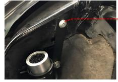
Remove one of the rubber mounts from the bottom of the OE airbox and press in to the rear airbox mounting hole in the chassis leg.
