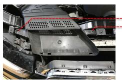
4 Unclip the intake ducting from the airbox and remove from the vehicle.
